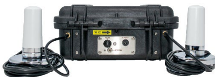
Fig. 3 (below): External coaxial connections.
