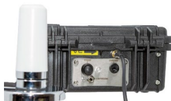
Fig. 3: External antenna connection.
