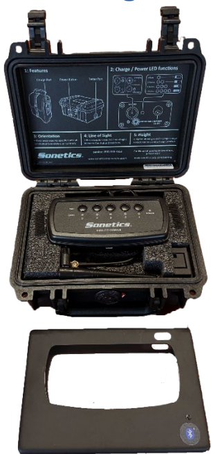
Fig. 1: Removal of faceplate.
